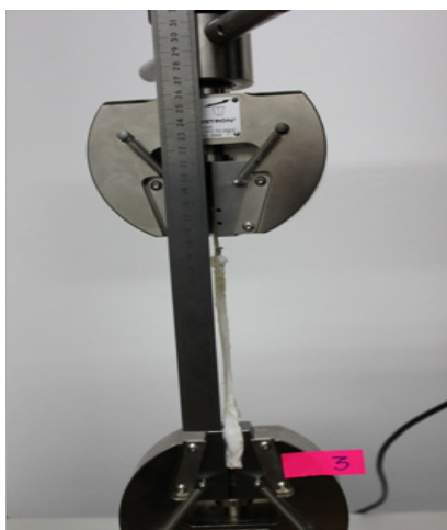
Figure 3. Construct fixed in testing device and measurements taken.
